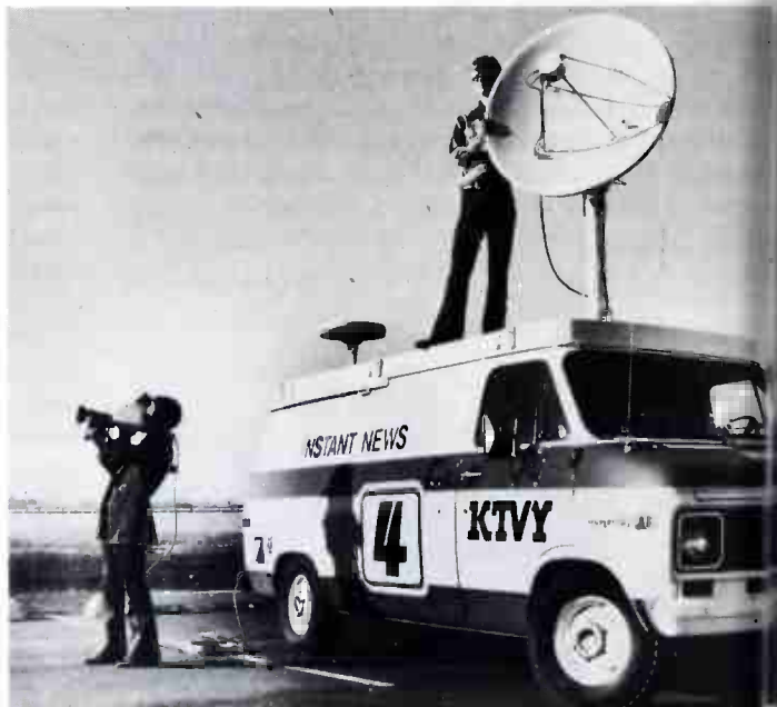
KTVY maintains an ENG crew for stories that need immediate air break. Shown is Fernseh KCN camera, truck with microwave link to studios. For field recording, truck carries Sony 3800 units.
